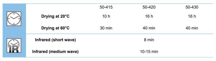
Please note: For automotive refinish, repair instructions of vehicle manufacturers, in particular regarding installed sensor technology, must always be observed in addition to the processing instructions given within this document.
